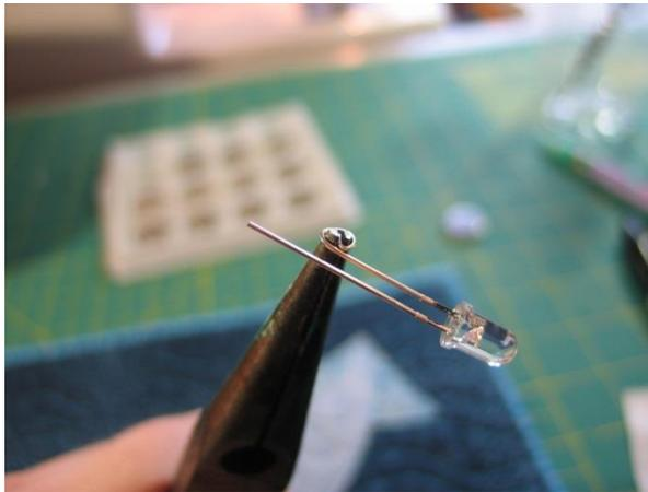
See how one leg of this LED is marked with the marker? That's the POSITIVE leg.
