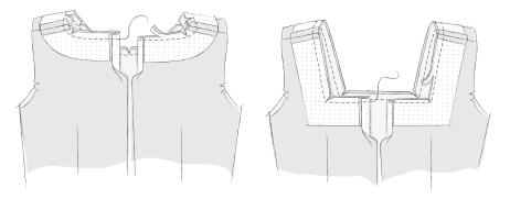
**3. Understitch neckline:** From RS, with facing/lining opened out from bodice and seam allowances underneath, stitch the facing/lining 1/8 in (3 mm) from seamline, catching seam allowances in stitching. Turn facing/lining to bodice WS and press neckline edge, rolling seamline inside.
