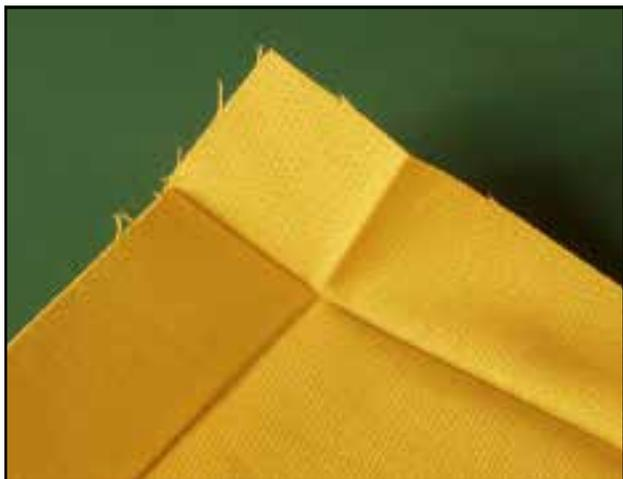
Fold the corner in toward the center at the point where the creases intersect. Match the crease lines within the corner to those of the square, creating a diagonal bias fold. Press lightly so that the bias is not stretched, but a crease line is created.
