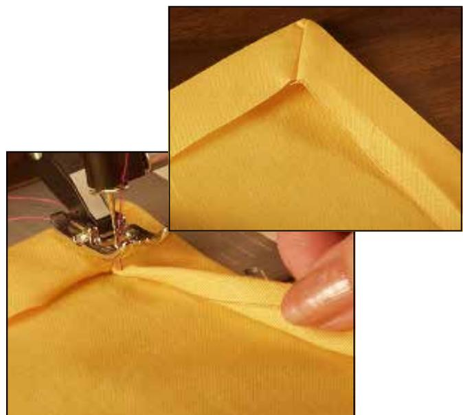
Finally, turn under a 1/4 inch hem and stitch a “needle width away” from the fold.
